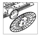
3. Push the LCD TV onto the base., Rotate the machine about 15 degrees according to the arrow on the base stand .
